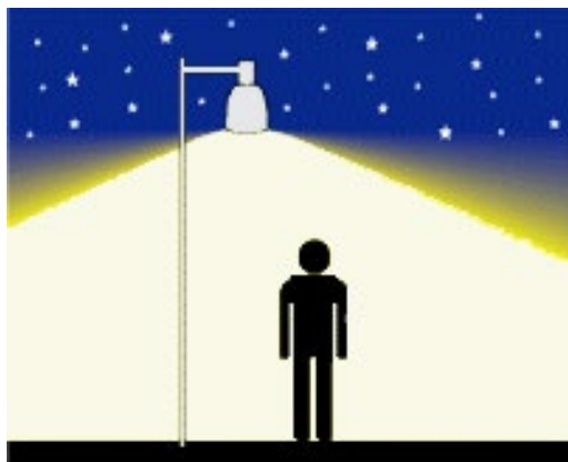
Figure 3, Full Cut-Off Lighting
