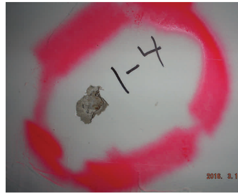
Sample 1-4 Plaster/Skim Coat
