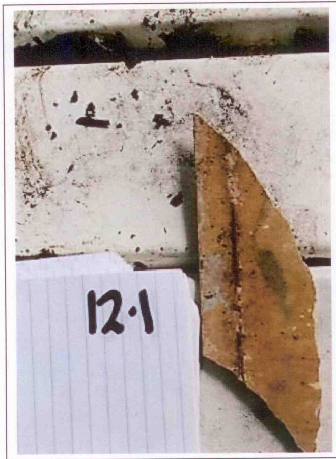
Brown mastic associated with 12" tan floor tile
