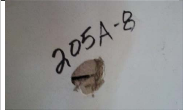
Photo 8: Plaster/Text. Pt. (205A-8) Bedroom 2, Wall C. Trace <1% Chrysotile Asbestos Detected (Base Coat) (PC=<0.25%).
