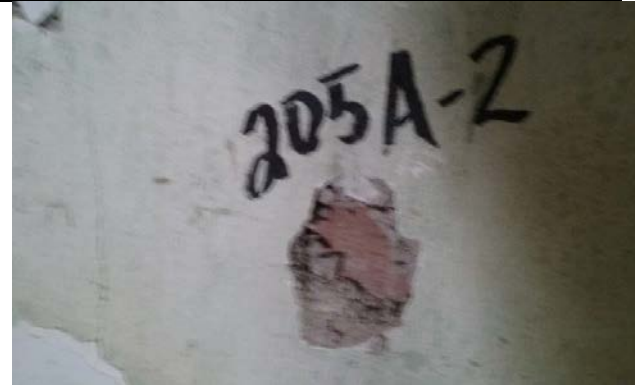
Photo 2: Plaster (205A-2) Living Room, Wall B. Trace <1% Chrysotile Asbestos Detected (Base Coat) (PC=0.25%).
