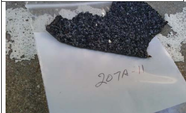
Photo 11: Roof Shingle (205A-11) Roof. No Asbestos Detected.
