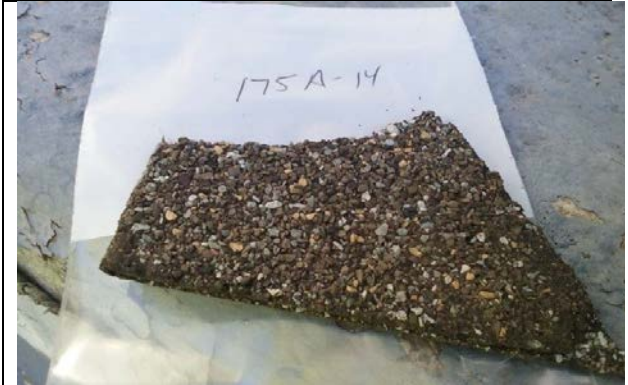
Photo 14: Roof Shingle (175A-14) Roof. No Asbestos Detected.
