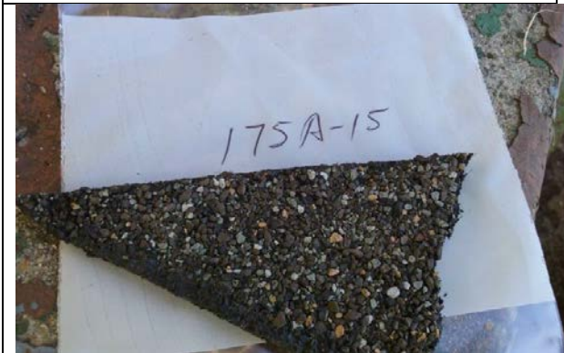
Photo 15: Roof Shingle (175A-15) Roof. No Asbestos Detected.
