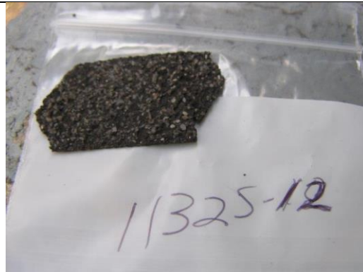
Photo 12: Roof Shingle (1132S-12) Exterior. No Asbestos Detected.
