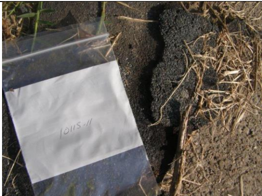
Photo 11: Roof Shingle (1011S-11) Exterior. No Asbestos Detected.
