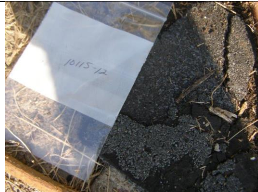
Photo 12: Roof Shingle (1011S-12) Exterior. No Asbestos Detected.
