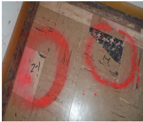
Sample 1-1 & 2-1, 9" Floor Tile/Mastic
