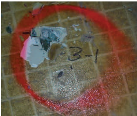
Sample 3-1 Linoleum/Leveling Compound
