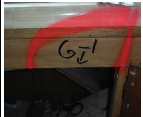
Sample 6-1 Sink Undercoating
