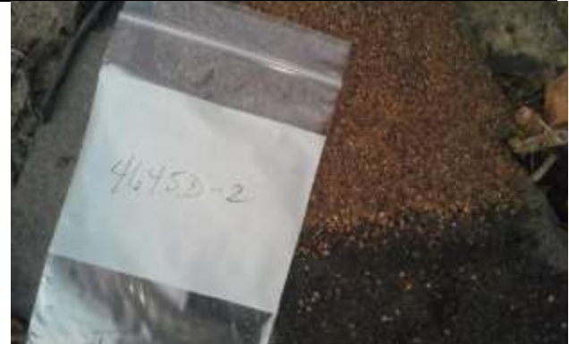
Photo 2: Roof Shingle (4645D-2) Roof. No Asbestos Detected.
