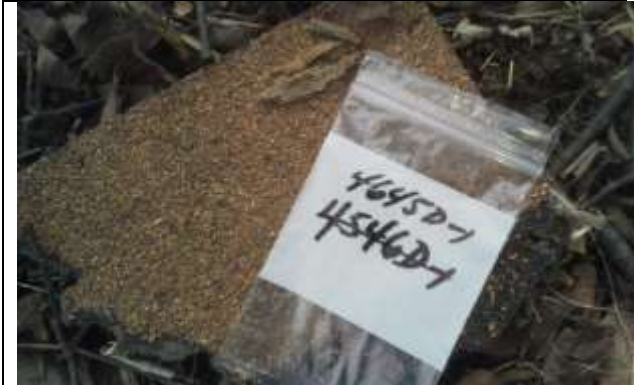
Photo 1: Roof Shingle (4645D-1) Roof. No Asbestos Detected.
