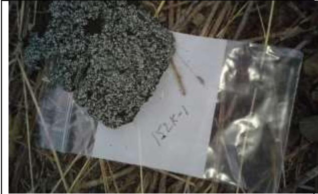
Photo 1: Roof Shingle (152K-1) Exterior. No Asbestos Detected.
